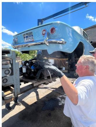
After lunch, the guys were ready to put the rebuilt 110 in the car. Pat pulled out the fork lift and the guys guided Pat as he skillfully got the engine in place so they could bolt it down. I was impressed with how Pat could move the pallet with the engine on it just an inch at a time in the direction the guys were telling him....'up two inches; to the right one inch,' and so on.
