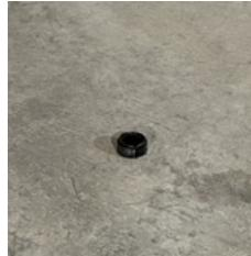
It’s not normal to see a universal joint bearing cap on the floor, so my interest was piqued at this. I pushed the car back into the driveway and jacked up the rear end to observe that one of the bearing cap retainers on the yoke was missing and the left universal joint was off the differential yoke. This is a big deal and I’m
