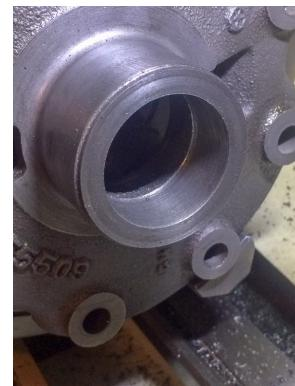
Step 3: Turn down the OD of the sleeve material (I chose chromoly tubing with a .188 wall thickness) so it is just a little bit larger than the ID cut in the carrier halves to make a good press fit.
