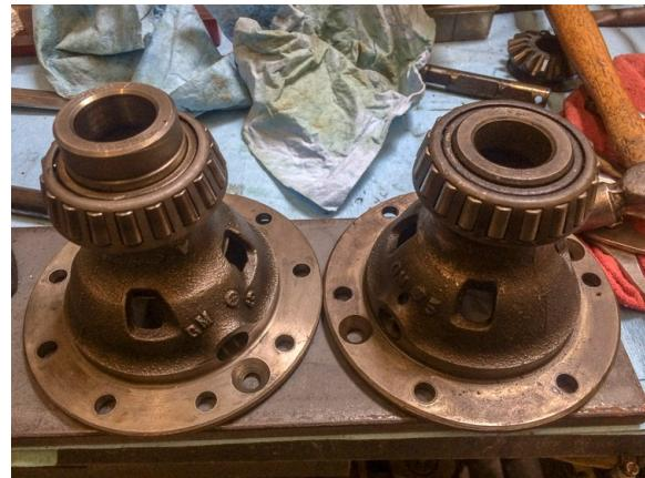
Early and late differential carriers sit side by side as a comparison of the differences between the two. Late parts are the taller, and also note the difference in the bolt pattern for the ring gear mounting.
