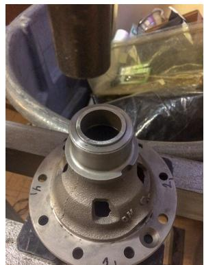
Step 5: Bore the ID to get a nice fit to the axle yokes (about .002 over), and trim off any excess sleeve material.
