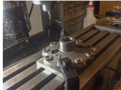
Step 2: We first need to bore out the ID of the carrier halves to allow the insertion of a steel sleeve. What turned out to be the biggest hassle, was to get the part centered in my 4 jaw chuck!
