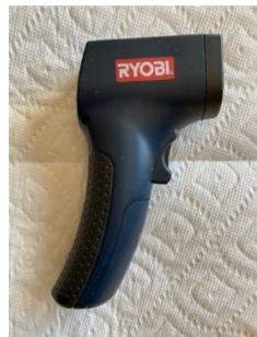
Non-Contact Temperature Reading Device
