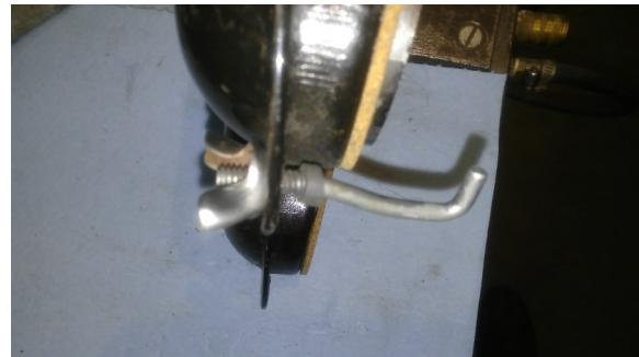
Early model cars/FC with the single air cleaners on each side should have a foam gasket for air cleaner top to carb air horn and generally those will stay with the air cleaner top. If the cork gaskets are used in place of the foam then using the above adhesive technique will work for those too.
