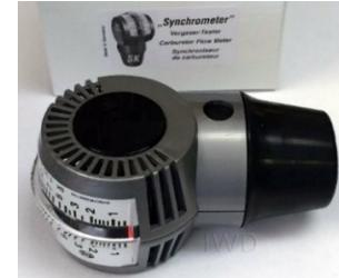
“Snail” Type Air Flow Measuring Device
