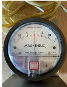
Magnehelic Null Reading Gauge (Dwyer Instruments)
