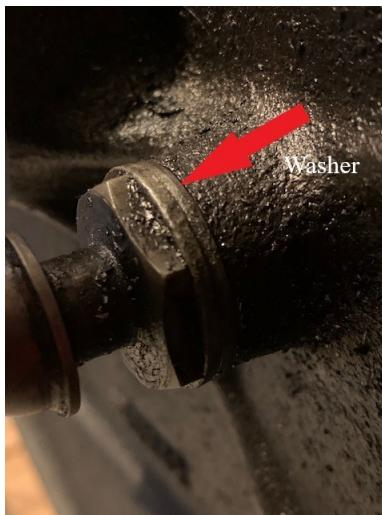
After removing the washer and putting the diff/transmission back together again, voila, the grinding was gone and there was some "play" in the clutch rod. Was definitely relieved the problem was solved.
