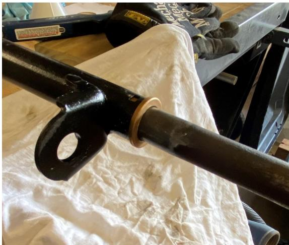
Well it turns out it does stretch enough. While I was down there, I replaced the accelerator linkage bushings and other deteriorated rubber. So, with the tunnel work done I moved to the dash.
