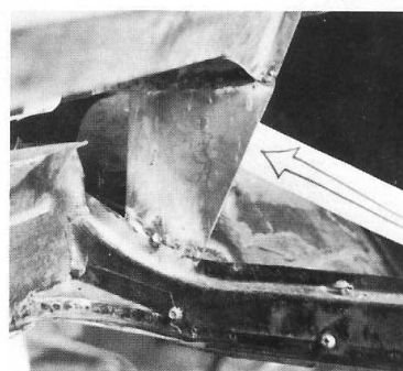
A brace was added to each side to support the rear deck lid hinge.
