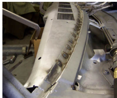
New Clark's Windshield Repro Panel. Body Man Even Took Time to Simulate Welds.
