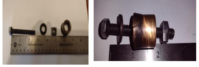
A hex head bolt, washer and square carriage nut were found in the spares and put together to be my forever tool. The Square 9/16th nut is narrowed on opposing flats to less than a half inch so that it may be inserted through and behind the pilot bushing. A reused washer with a hole smaller than the bolt head is placed on the bolt after the nut is in place and before the is bolt started into the threads of the nut..
