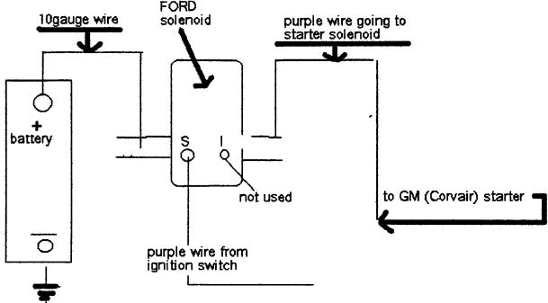
the purple wire coming from the ignition switch to the GM starter solenoid is split apart at the small plug in the engine bay. The wire coming from the switch is attached to the 's' terminal on the FORD solenoid. This wire has the effect of 'throwing the switch' inside the FORD solenoid, connecting the voltage from the battery directly into the GM solenoid.
